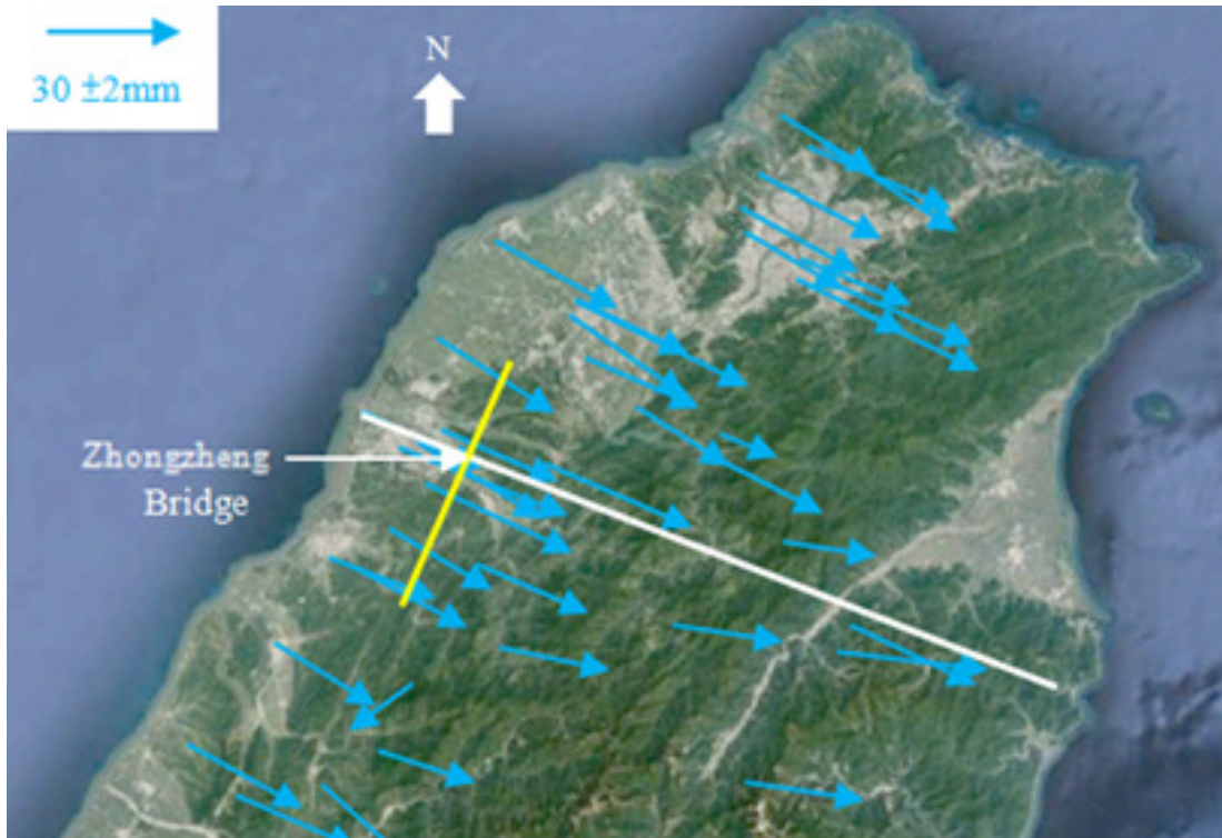
Figure 20. Shear bands identified from the GPS velocity-vector distribution map (background image from Google Earth, 2020, and GPS velocity vectors from GPS LAB, 2007).
