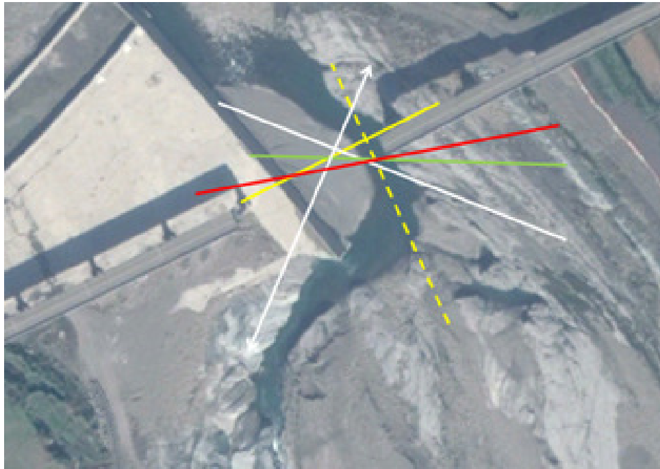
Figure 22. Shear bands that induced the collapse of the Zhongzheng Bridge (background image from Google Earth, 2020).
